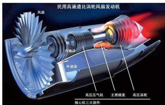
Figure 1. Turbine engine with high bypass ratio for civil use scheme
