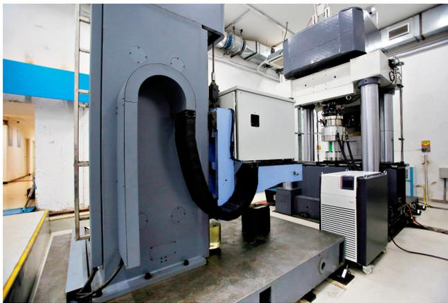
Figure 1. In-situ geomechanical testing facility featured by high energy linear accelerator CT scanning and multi-field coupling
