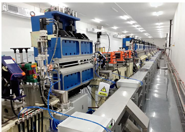
Figure 2. High order harmonic amplifier of Dalian Coherent Light Source
